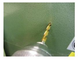
Drill a hole  $\emptyset$  6.8 mm and make M8-threadings for the fastening screws.
