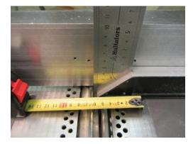
Make a mark on the side stopper along the centre line of the blade. This eases the task of installing the protector so that it is in the middle of the blade line.
