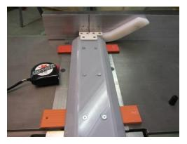
Making use of the mark you made earlier, place the protector so that it is in line with the centre line of the blade.
