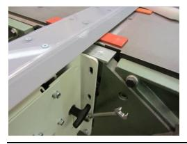
Ensure that the protector remains straight when tightened.
