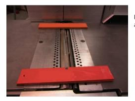
Place the plates provided with the protector (in the package they are white, and not as shown in the diagram) onto the worktop as shown in the diagram.
