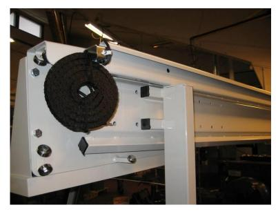
Push the shavings protector from the tailstock side onto the guide rail. When doing so, place also the energy transfer chain onto the C profile you just installed.
