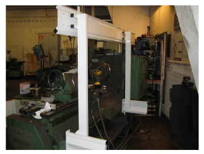
Fasten the guide rail by means of screws to the upright pillars kruva fast styrskenan i de lodräta stolparna.
