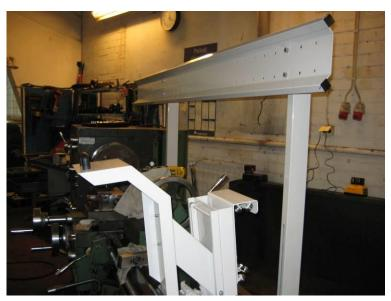
Adjust the guide bar so that it is straight. Begin the installation of the chuck protector and its micro enclosures.
