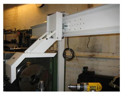
Place the chuck protector onto the guide rail.
