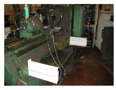
Begin the installation by locating and fastening the horizontal brackets.
