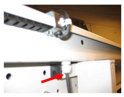
Drill a lead-in (Ø 13 mm) for the power cable at a desired location along the lower edge of the C profile. Put in place and tighten the cable clamp.
