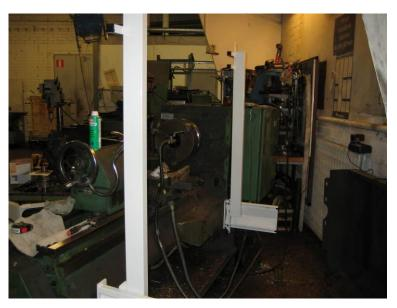
Fasten the angle bars to the upright pillars' grooves (using flat nuts inside the pillar). Fasten the upright pillars to the horizontal brackets by means of the flat nuts in the C profile.
