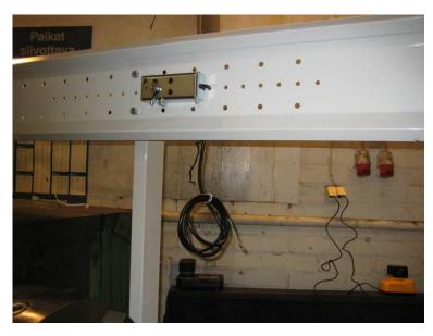
The right-hand edge of the micro enclosure needs to be at the same level as the chuck protector's right-hand edge. Ensure that the micro enclosure's right-hand edge does not go beyond the chuck's jaws. The washers in the bag are meant to be placed between the guide rail and the micro enclosure. Fasten the micro enclosure by means of screws to the guide bar.
